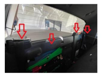
Remove the driver's side child seat anchor mount (10mm socket) and seat retaining tab (T40 Torx) Remove Plastic clips holding carpet on the back wall. Retain all components.
