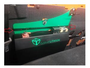
9. With help of a friend, lift the battery into place with the lower locating pin picking up the hole in the jack mount. The 4 mounting holes will then realign to the child seat anchor point and rear seat locking plate. These items will then be refixed using the original bolts. If using the Ausmotion DCDC mount, follow instructions for fitment. (If the pin at the bottom of the battery appears loose, you can use a nut to thread onto the pin and tighten it into place)
